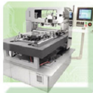
NexTech FAS Advantage slot coaters are available for substrate sizes through 6m & and feature 95% material utilization.
